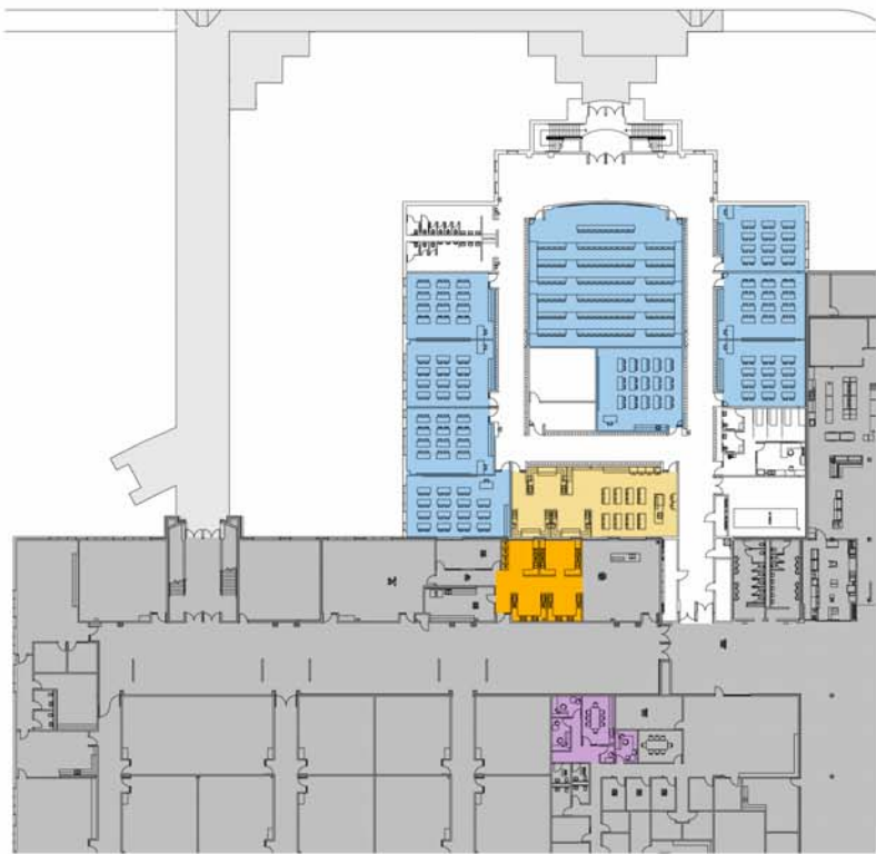
classroom addition first floor plan not to scale addition per floor: 22400 sq. ft.
